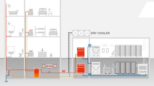
Because of the high condenser leaving water temperature, EW-HT-C enables data centers to reuse exhausted heat for wide applications, resulting in having more chance to achieve higher ERF than lower temperature
